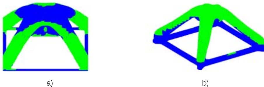
Fig. 10: Optimal topology: (a) SESO; (b) VLSM (present formulation)
