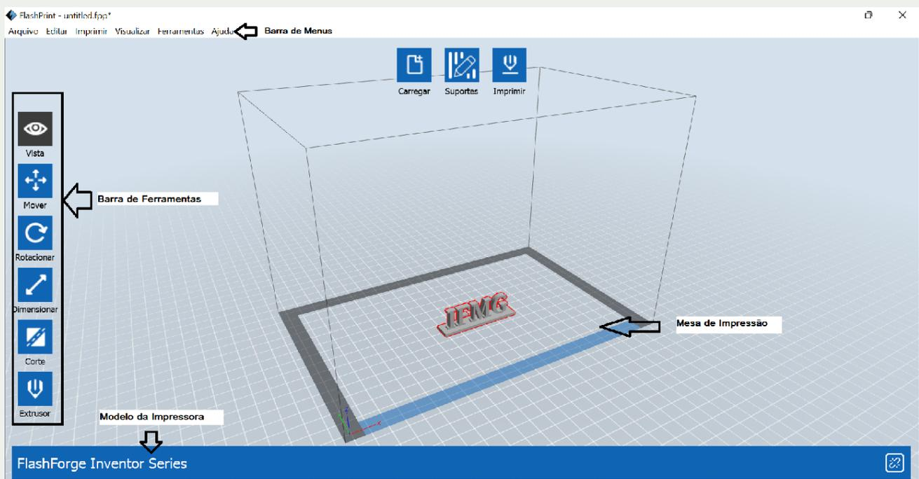
Figura 8: Interface do Software FlashPrint v4.6.4
