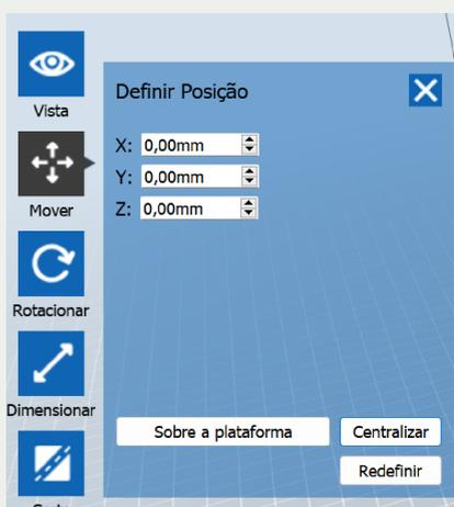
Figura 14: Ferramenta Mover no Flashprint
