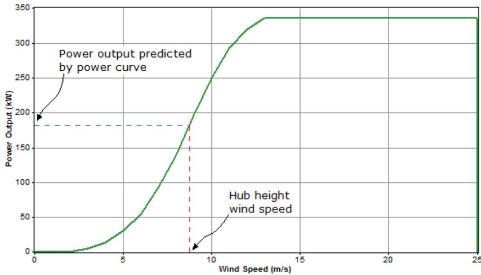
Figure 11. Wind turbine curve (output x wind speed) [21]
