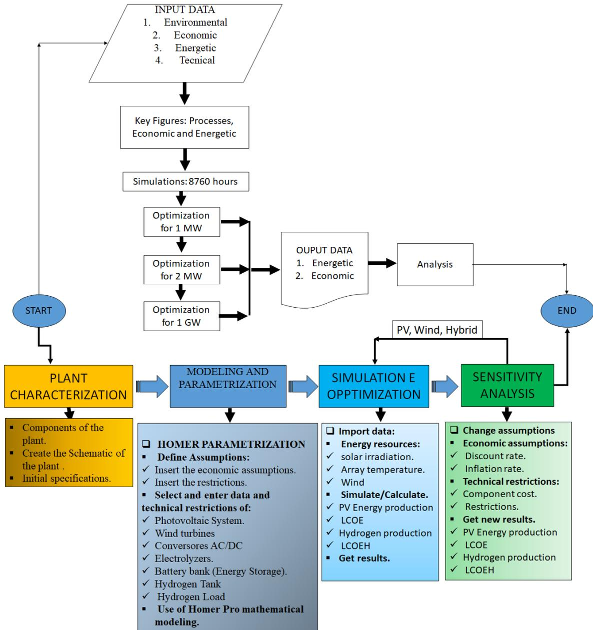
Figure 9. Flowchart of the dynamic simulation and optimization method, adapted from [24]
