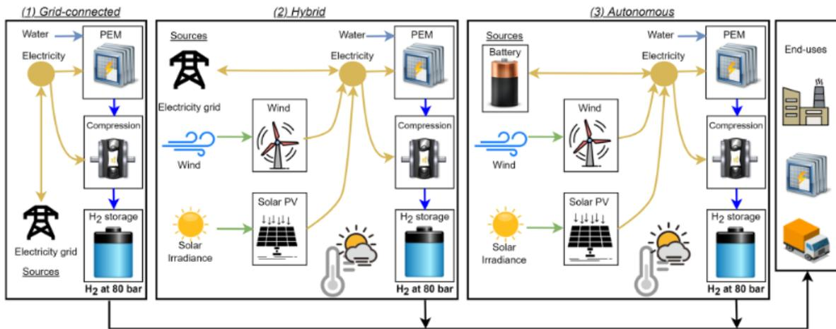
Figure 3. Hydrogen production configurations on grid, hybrid, and autonomous [18]
